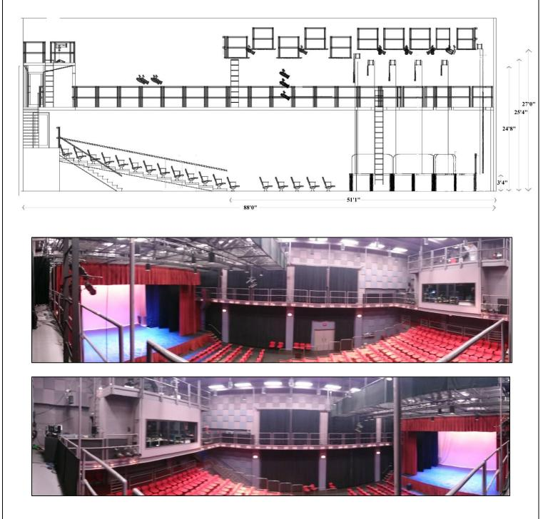
The control booth is located 84' from the back wall and is level to the catwalk. It contains the lighting control console, stage manager desk, and front projection control. The sound console is located on the catwalk to the house right side of the control booth.
